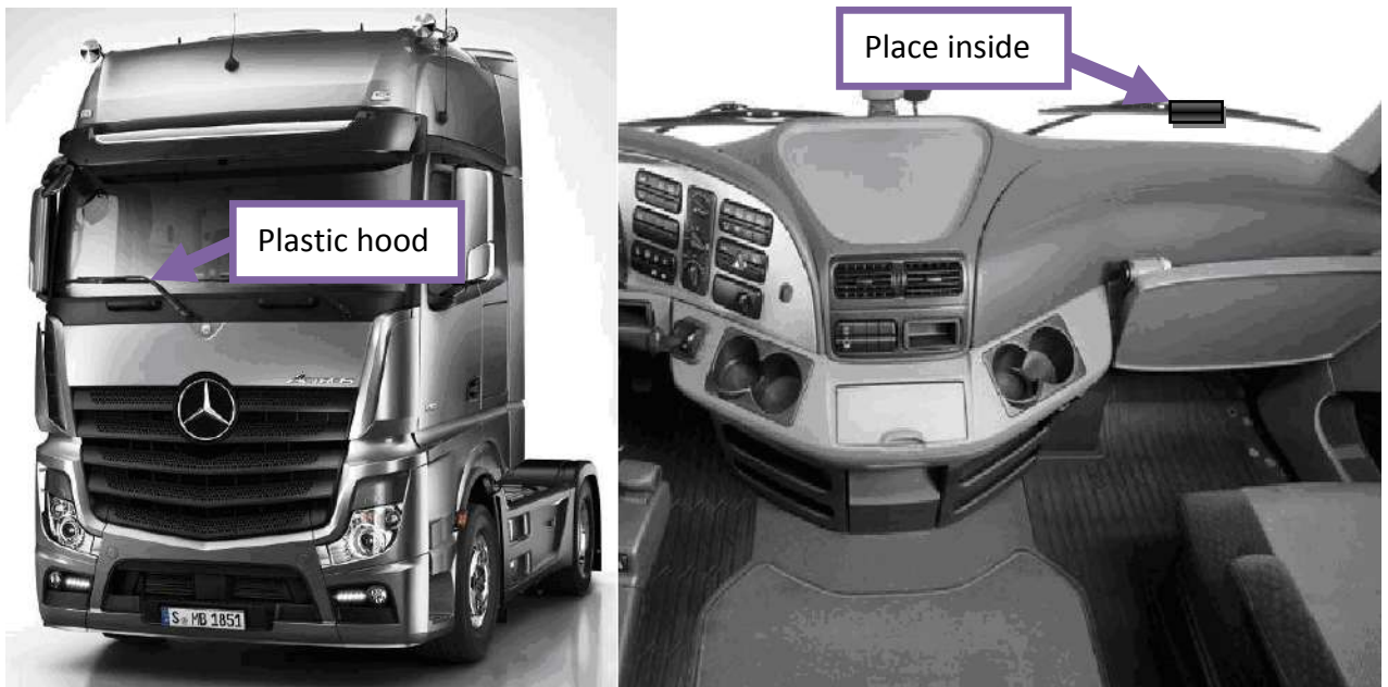
Figure 58. Possible mounting places in trucks
